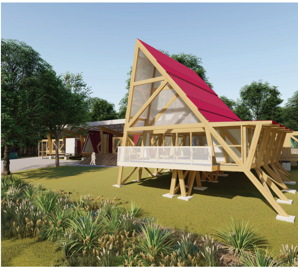
Community Hall: Prefabrication for Transport and Adaptive Reuse Three sets of trusses are transported, stacked, and clipped together.
